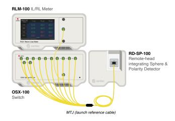
Step 2. Connect the DUT then measure Polarity,  $\rm IL_{A}$  and  $\rm RL_{\Delta}$
