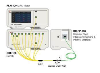
**Step 3**. Flip the DUT then measure  $IL_{R}$  and  $RL_{R}$
