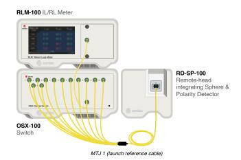
**Step 2**. Connect the DUT and the receive MTJ then measure Polarity,  $IL_{Total}$ ,  $RL_A$ ,  $RL_B$  and  $RL_{Total}$
