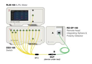
Note: you can configure the test plan to check polarity before IL/RL to get a quick pass/fail on polarity in the first few seconds. If polarity is good, the software automatically continues without any operator intervention. This fast fail method makes your testing efficient, so you don't waste time measuring IL/RL on a cable with incorrect mapping.
