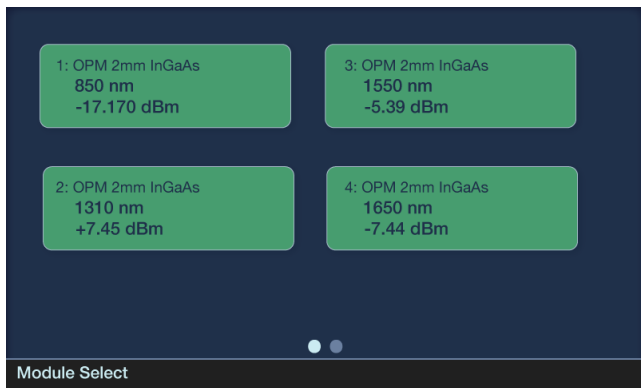
Figure 2: Front panel of OPM-200 power meter with 4 power levels displayed simultaneously.
