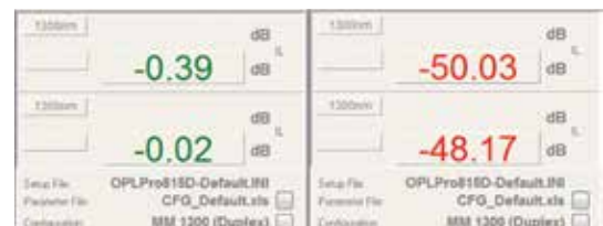
Figure 6: Above shows two values: one passing and one failing. The passing values verify that the DUT passes for both IL and polarity. The dark values (right) show that the cable is failing whether it's by broken cables or incorrect polarity.
