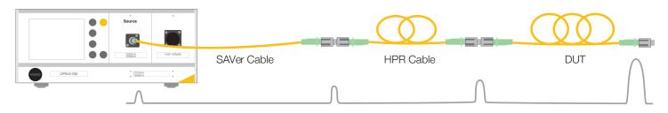
By leaving a SAVer cable attached to the front panel of a unit, interface damage can be avoided, preventing downtime and minimizing repairs costs.
