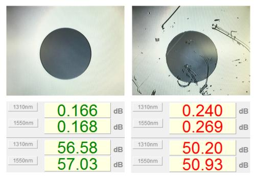
Dirt and damage can greatly affect not only the visual qualification of a cable, but also its insertion loss and return loss.
