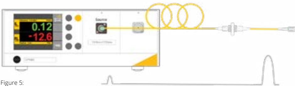
Figure 5: With no receive cable connected to the short DUT, the reflections of the unterminated end overpowers the smaller reflection.
