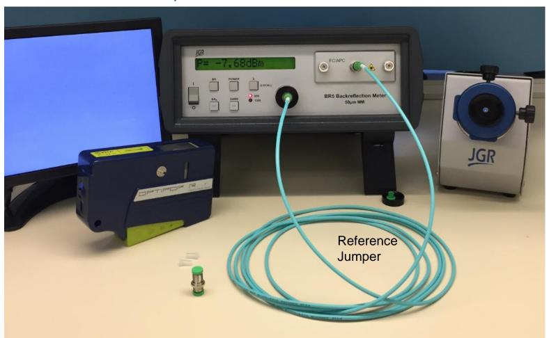
• Press and hold the "POWER" button until a click can be heard. Once the button is let go the meter will read "0.00dB rel" as shown below.
