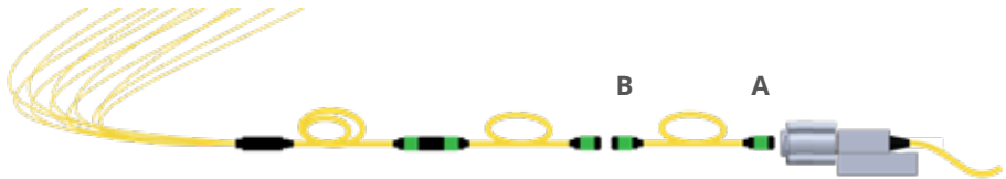
Figure 31 - Side B is tested on the second breakout cable corresponding to its gender.
