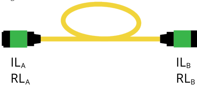
Figure 38 - The standard method yields connector-level results for IL and RL.
