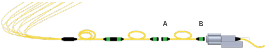
Figure 30 - Side A is tested against the correctly gendered launch cord.
