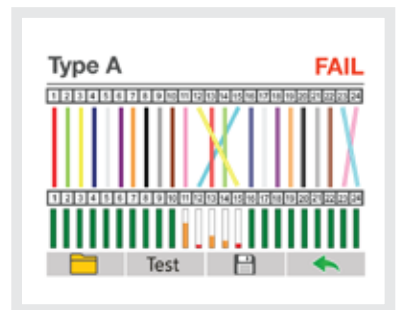
Figure 25 - Passing and Failing Polarity Verification on the OP415.
