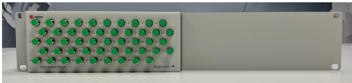
Figure 5: 2U half rack OSX-100 rackmount ear front view
