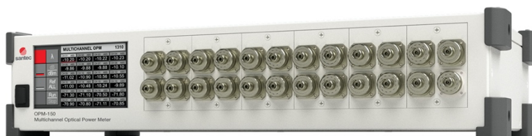
Figure 1: OPM-150 Multichannel High-Speed Optical Power Meter
