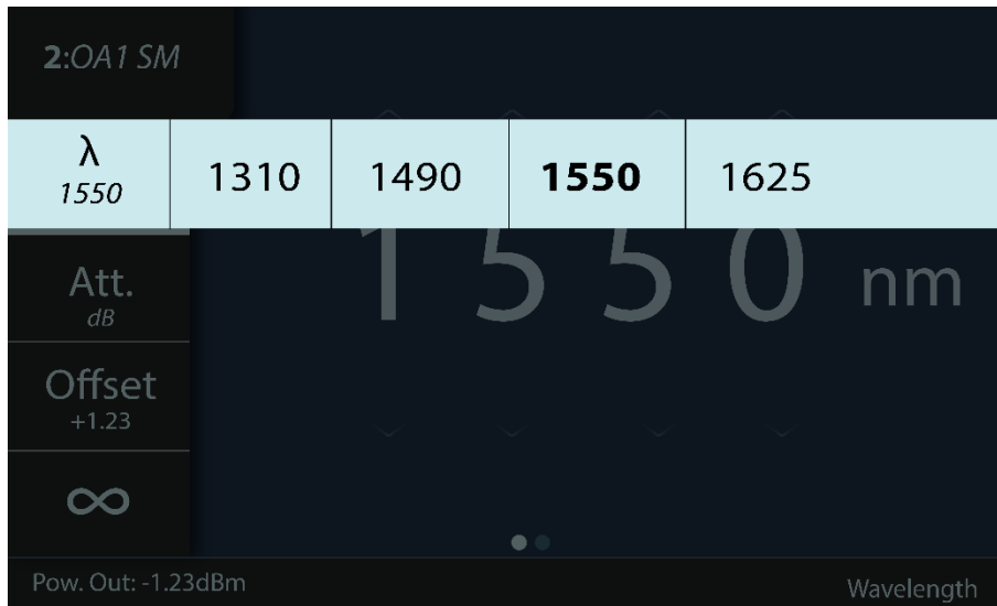
Figure 5: Front panel operation – wavelength flyout menu
