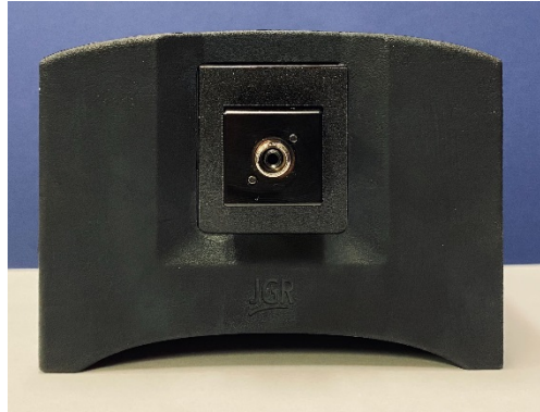
Figure 4: Front view of an RD-S with an SD01 slide FC detector adapter
