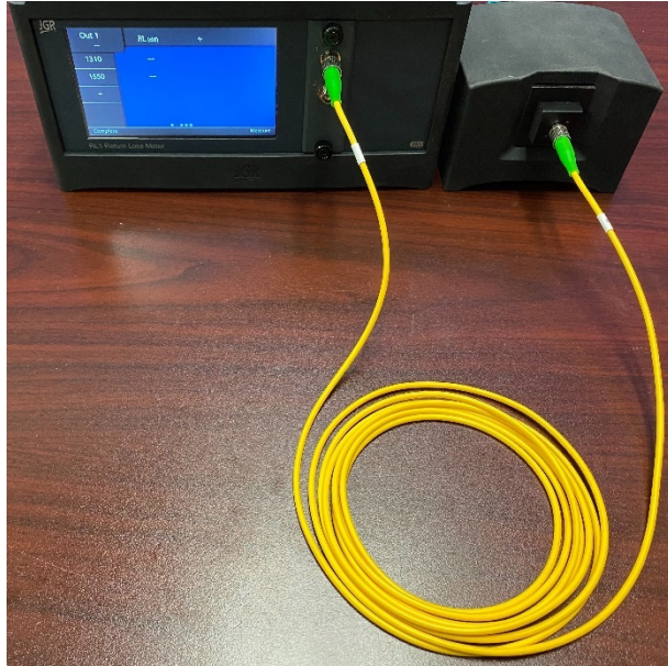
Figure 24: Example of good test jumper fiber management
